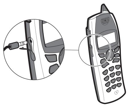
Plug the headset into the jack located on the left side of the handset (under the rubber flap). Please do not force the connection, but make sure the plug fits securely.
